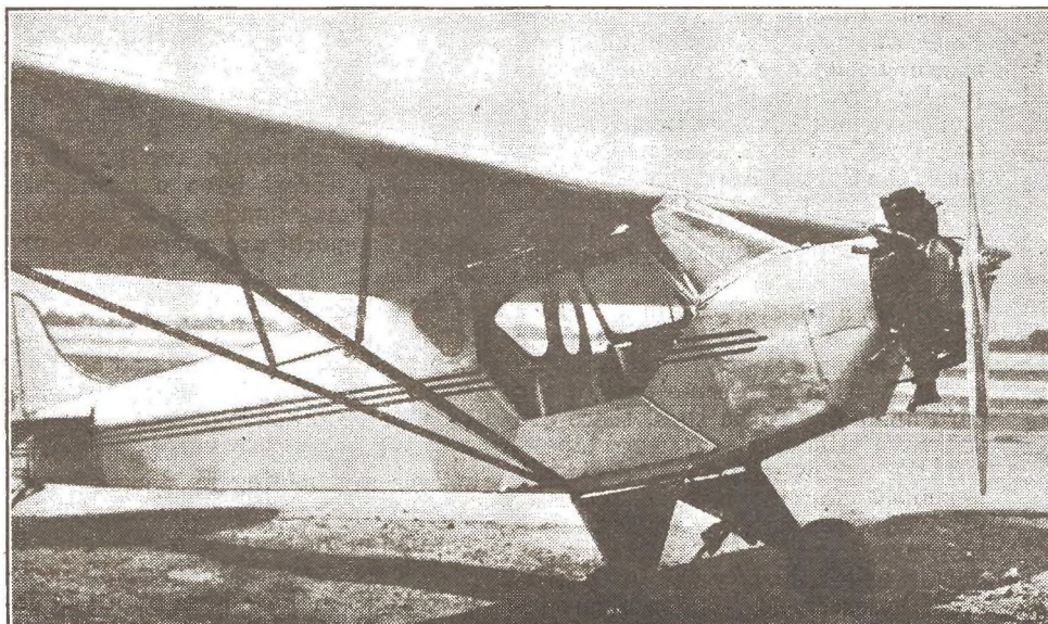
Left: Here's a close-up shot of the Piper Cub sporting the new 5-cylinder, 65-h.p. Angle engine. The interesting feature of this plant is that the cylinders and crankcase are cast in a single piece, and the whole motor is said to boast unusually light weight. We'll bet many a flyer will angle for an Angle-powered Cub!
